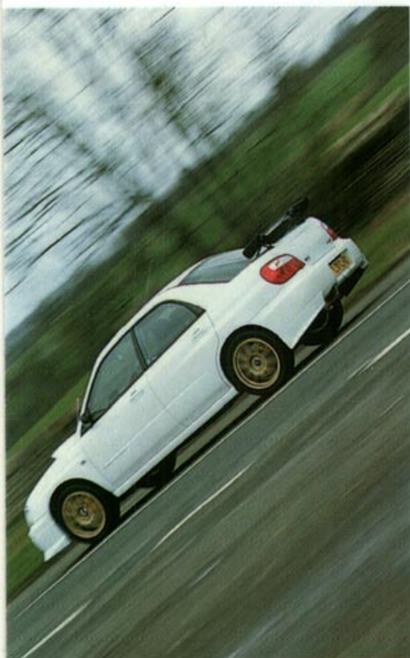
Spec C gets 322bhp and 325lb ft; rear wing now made of carbonfibre
