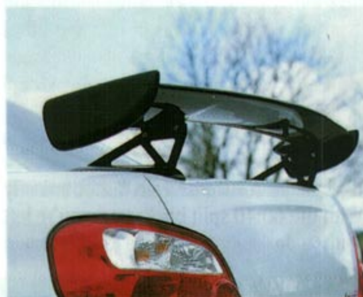
Spec C gets 322bhp and 325lb ft; rear wing now made of carbonfibre
